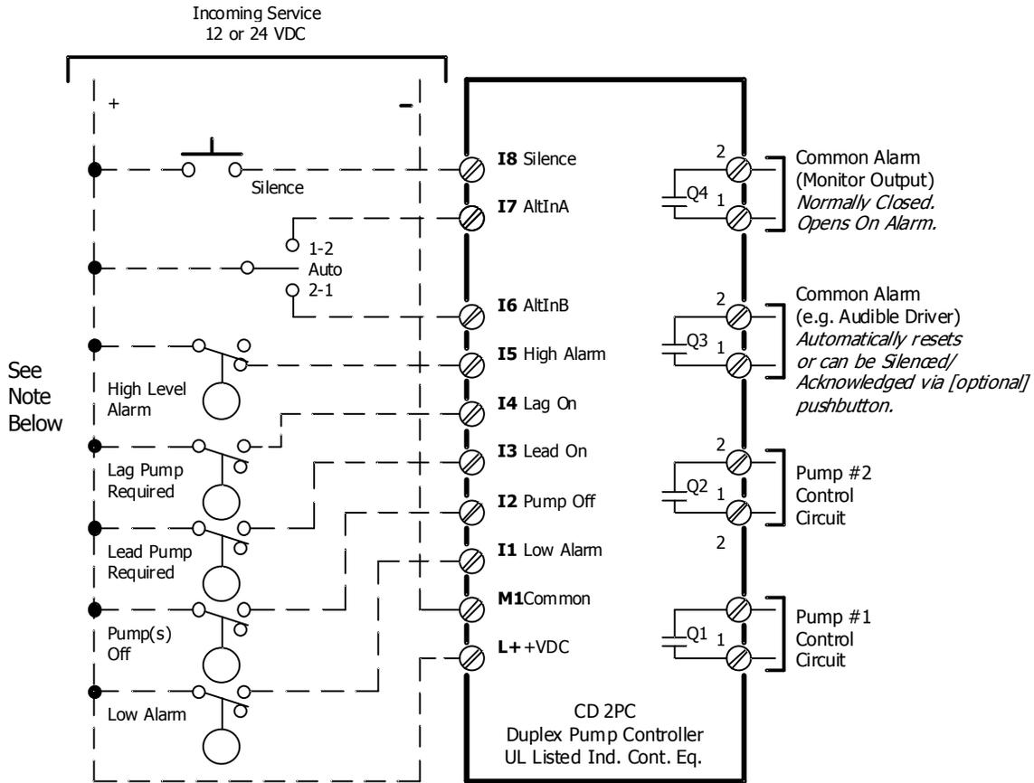
Note: The CD-2PCc can accept either a Normally Open (NO) or Normally Closed (NC) high alarm input. The controller's internal software switch must be set for the selected input type.
