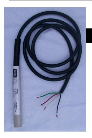
CONTEGRA'S SW 108 is a rugged, versatile tilt switch. The SW 108 was designed to provide pump discharge flow sensing for pumps which use a check valve arm. The SW 108 is fastened directly to the arm (as shown on page 2). When the check valve opens and the valve arm tilts upward, the switch toggles, signaling pump flow.
