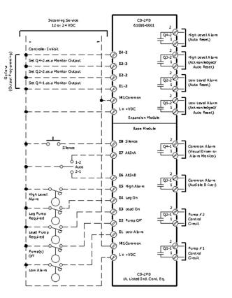
Duplex Pump Control w/Common High and Low Level Alarm and Independent High and Low Alarm Outputs
